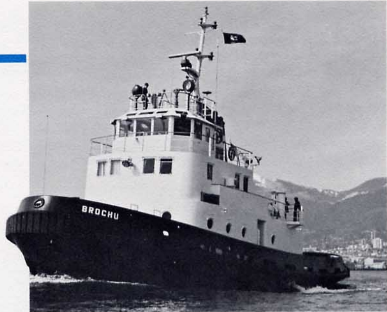
Special duty tug equipped with two 1,800 hp Model 251 engines berths iron ore carriers
