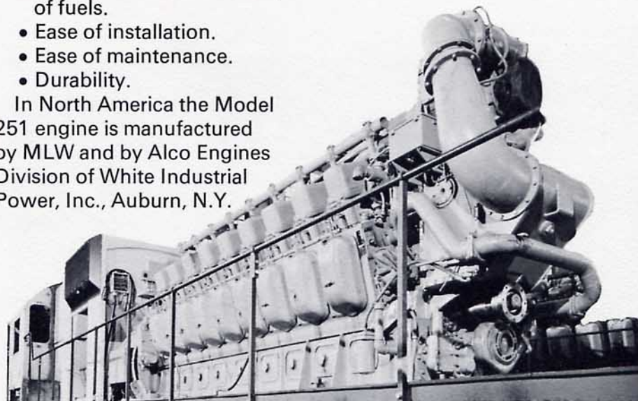
4,500 hp (4563 CV) 18-cylinder engine installed on locomotive chassis
